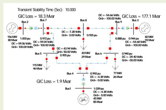
Nine bus system used to demonstrate a rapid, GIC induced voltage collapse
