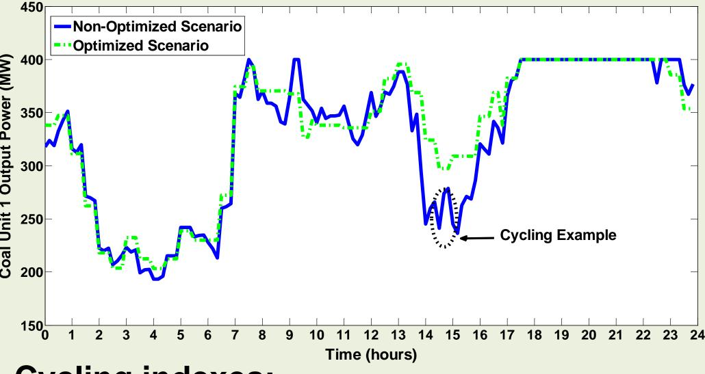
•Dispatch of a coal unit in the test system with 10% wind integration for optimized and non-optimized scenarios.
