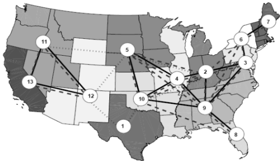
Fig. 4. Reduced national interconnection overlay. Existing HVAC (solid), HVAC overlay (dashed), HVDC overlay (dotted).
