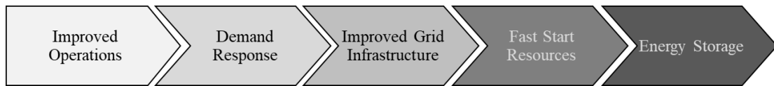
Figure 1.2 Cost comparison between different options to improve operational flexibility from lower cost on the left to higher cost on the right [24].
