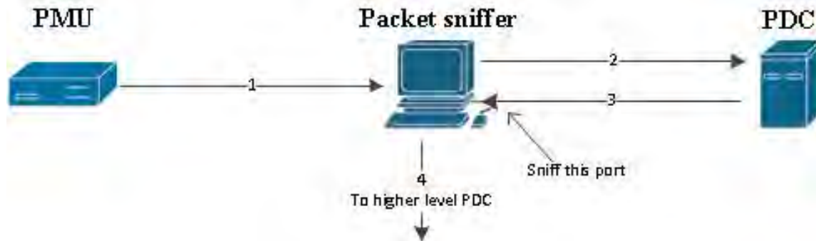
Figure 3.4: Network configuration for data processing time management.
