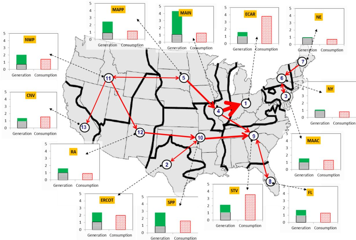
Figure 5: Illustration of transmission capacity needs for a renewable-heavy generation portfolio
