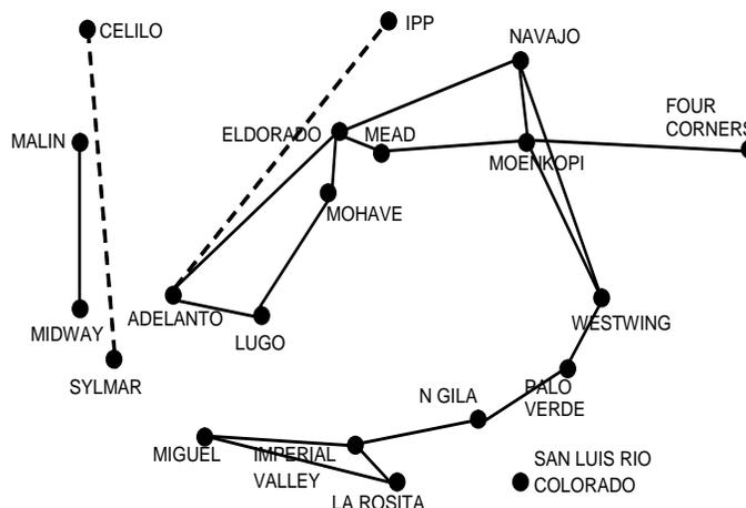
Figure 3: Stylized, simplified southern portion of the Western interconnection in North America. Dotted lines are existing HVDC lines. Solid lines are AC. Note that San Luis Rio Colorado and La Rosita are in Mexico. The PDCI is shown dotted (Celilo–Sylmar).
