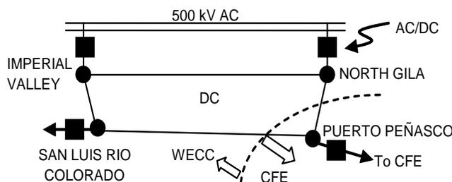
Figure 4: Simplified schematic of a meshed HVDC network joining WECC and mainland CFE (Mexico)
