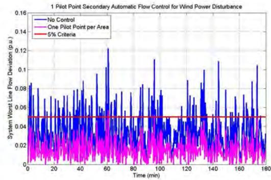
Fig. 17. The Effect of AFC on Line Flow Deviations in response to Wind Power Disturbances
