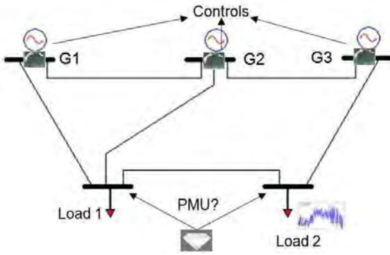
Fig. 1. Simple 5-Bus Power System with AVC
