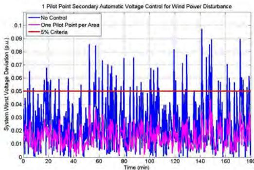
Fig. 16. The effect of AVC on Voltage Deviations in Response to Wind Power Disturbances
