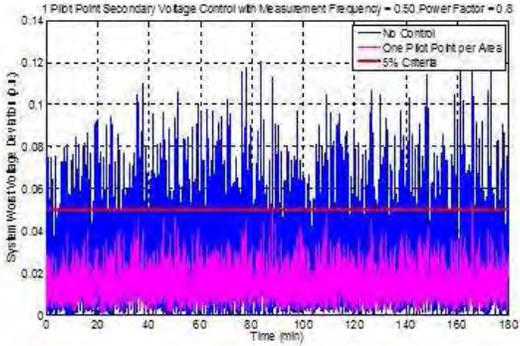
Fig. 8. Effects of AVC Control on NPCC voltages; High Power Factor Case
