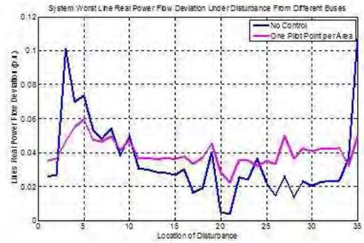
Fig. 14. The Worst System-Wide Real Power Line Flow Deviation Caused by Disturbances at Different Buses
