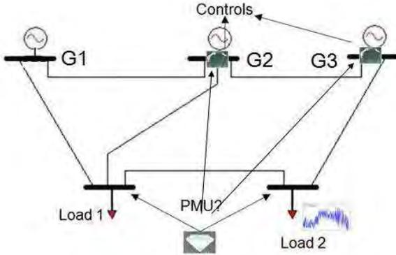
Fig. 12. Simple 5-Bus Power System with AFC
