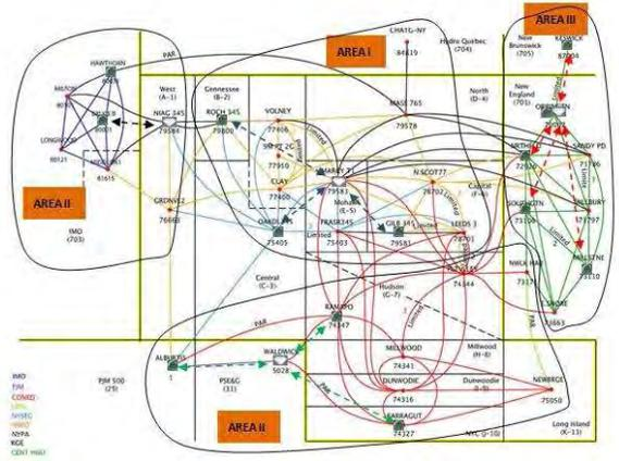
Fig. 13. NPCC power system with 4 control area implementation of AFC
