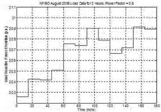
Fig. 5. 3 Hour Ahead Reactive Power System Load Forecast
