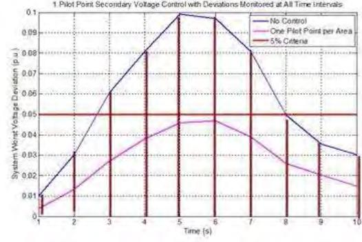
Fig. 10. Effect of Control with Fast Measurements
