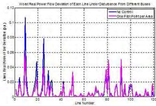
Fig. 15. The Worst Real Power Line Flow Deviation of Each Line under All Tested Disturbances
