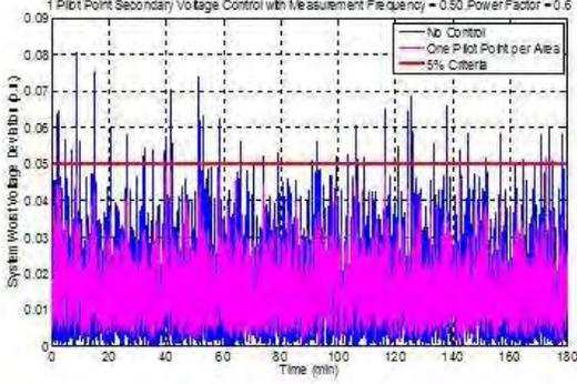
Fig. 7. Effects of AVC Control on NPCC voltages; Low Power Factor Case
