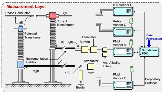
Figure 3. Conceptual Illustration of the SuperCalibrator with Dynamic State Estimator
