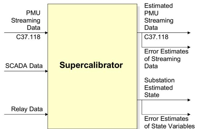
**Figure 1. Inputs and Outputs of the SuperCalibrator**
