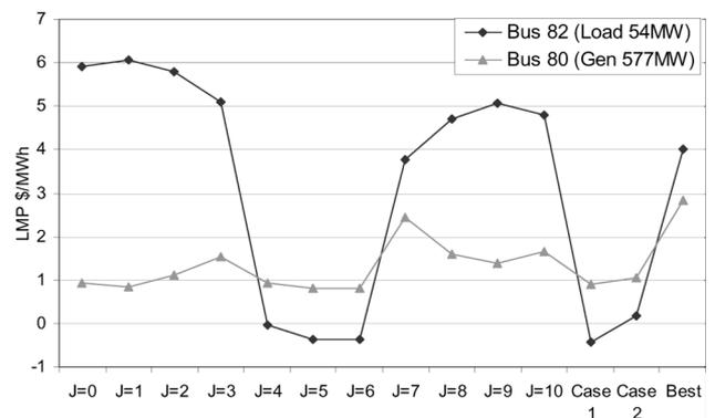
Fig. 4. Dispatched generator and load bus with largest LMP variance. The buses with the largest variance (mean square deviations) in LMP for these two categories are displayed.
