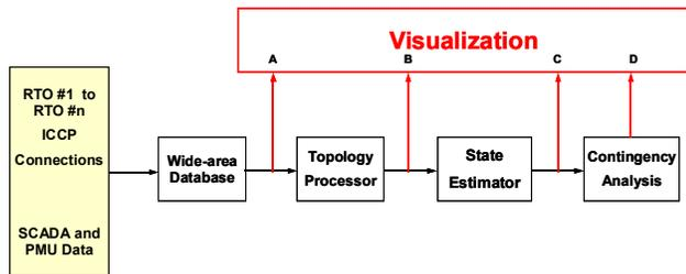
Figure 2: Schematic of the Wide-Area Analysis and Visualization Environment.
