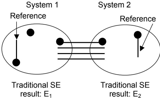
Figure 3: Concept of combining state estimates using phasor measurements.
