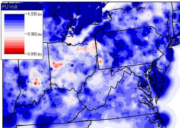
Figure 8: Pre-Blackout Ohio Region 115-230 kV Voltage Contour
