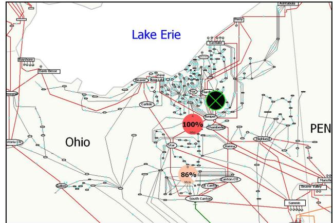
Figure 5: Northeast Ohio Transmission System Status after Loss of First 345 kV Line at 15:05 EDT
