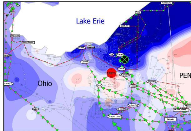
Figure 9: Northeast Ohio Voltage Contour at 15:05 EDT
