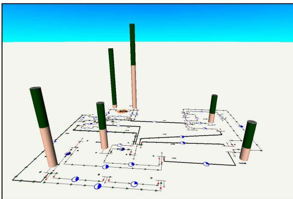
Figure 10: 3D View of 30 Bus System
