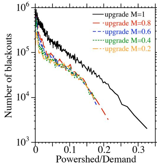
Fig. 7. The number of large blackouts as a function of blackout size for various operating limits  $M_R$ . The overall decrease in the number of blackouts is much larger for the first 20% increase in margin.
