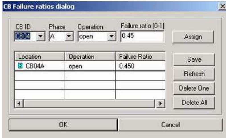
Figure 3.9 Dialog for setting circuit breaker failure ratios
