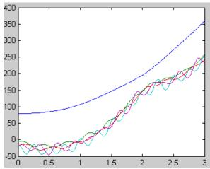
Fig. 7. Machine angles when 5.5% load shedding at t=0.11s
