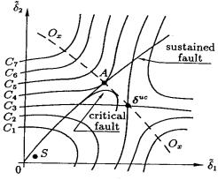
Fig. 2. System trajectory in the rotor angle space
