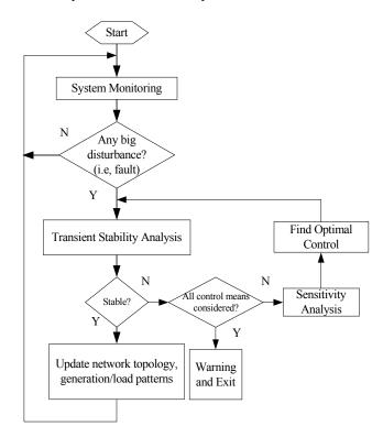
Fig. 3. Flow chart of the stability control scheme
