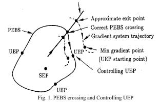
Fig. 1 gives the relationship among unstable equilibrium point (UEP), PEBS crossing point, exit point, Controlling UEP [4]. Fig. 2 gives a simple example of the system trajectory in the rotor angle space [5].
