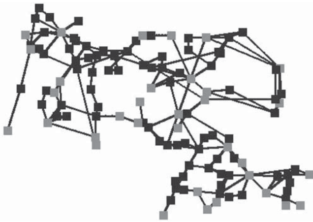
FIG. 1. Diagram of the IEEE 118 bus network. Generators are gray squares; loads are the black squares.
