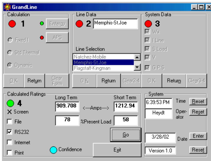
**Figure (4) A graphic user interface for the calculation of a real time rating of an overhead transmission circuit based on sag**
