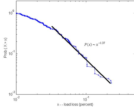
**Figure 13. Power law “tail” of simulated DC power loss time series in constant-load model**
