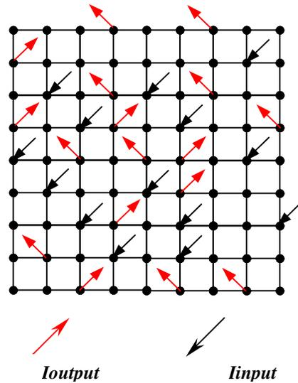
**Figure 9. The fuse model of simplified power network**
