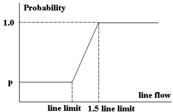
**Figure 10. Probability of an exposed line tripping incorrectly**
