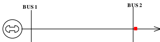
Figure 6.7 The two-bus system
