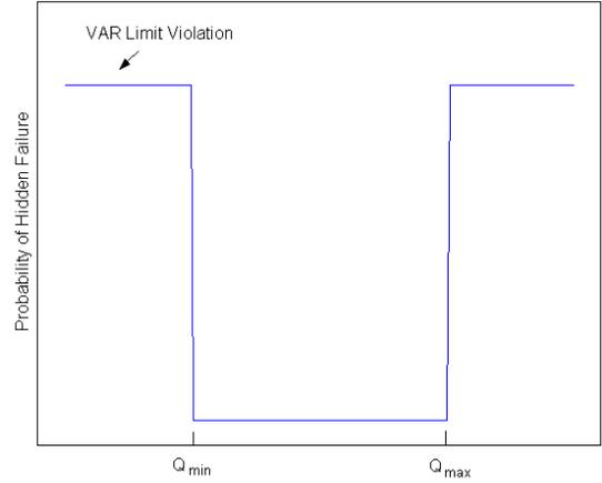
Fig. 3. Probability of hidden failure in generator protective relays
