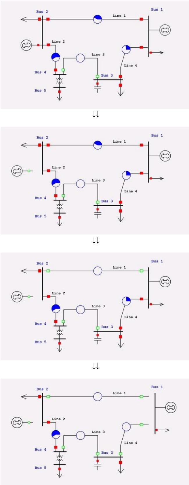
Fig. 4. Evolution of the power system during disturbances
