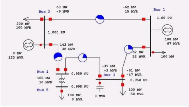
Fig. 1. Illustration of key equipment in a 5-bus system
