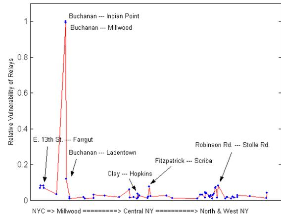
Fig. 6. Locations of most vulnerable relays in NYPP
