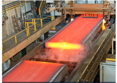
(b) Cutting a slab from the strand exiting a continuous-caster [Primetals Technologies, 2019]
