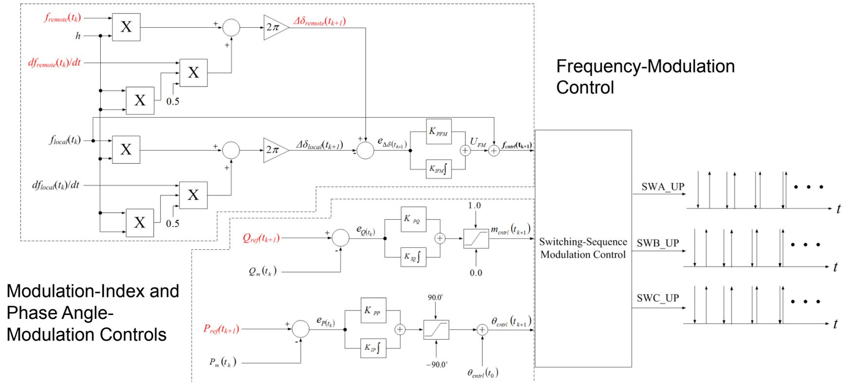
The frequency-modulation control **gradually** modulates the frequency of converter switching sequences to slowly synchronize with remote-end transmission and prevent large current transient. The modulation-index and phase-angle modulation controls modulate the amplitude and phase angle of the AC output voltage by controlling the duty ratio and start time of switching sequences.
