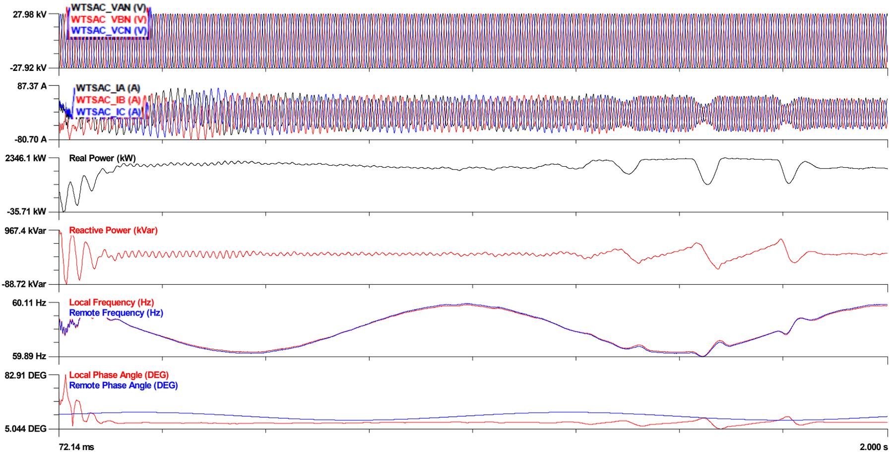
We perform this simulation test for a case that a remote converter-interfaced generation (CIG) is under frequency oscillation when a local CIG does not have the Predictive Inverter Controller. The frequencies of two CIGs cannot synchronize with each other, consequently power-factor angle difference oscillates. Thus the CIG systems exceed their desirable operation constraints. Therefore, CIG system requires the Predictive Inverter Control to minimize the transient.
