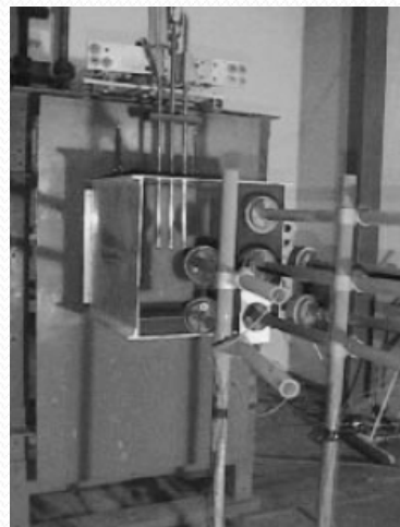
3Φ Arc-in-the Box Test Setup
